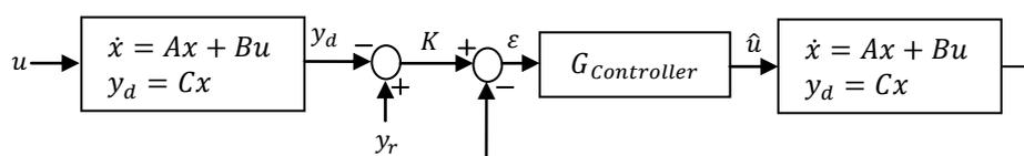
Fig. 1. The architecture of the proposed disturbance estimator
