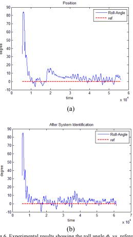
Fig.6. Experimental results showing the roll angle  $\phi$  vs. reference 0° with empirical PID coefficients (a) and PID coefficients tuned on the identified model (b).
