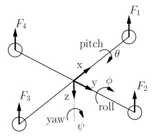
Fig. 1. Simple Quadrotor Model
