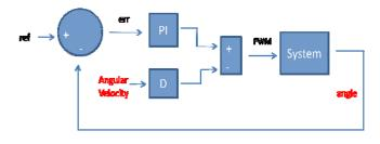
Fig. 4: Block diagram of the PID Controller
