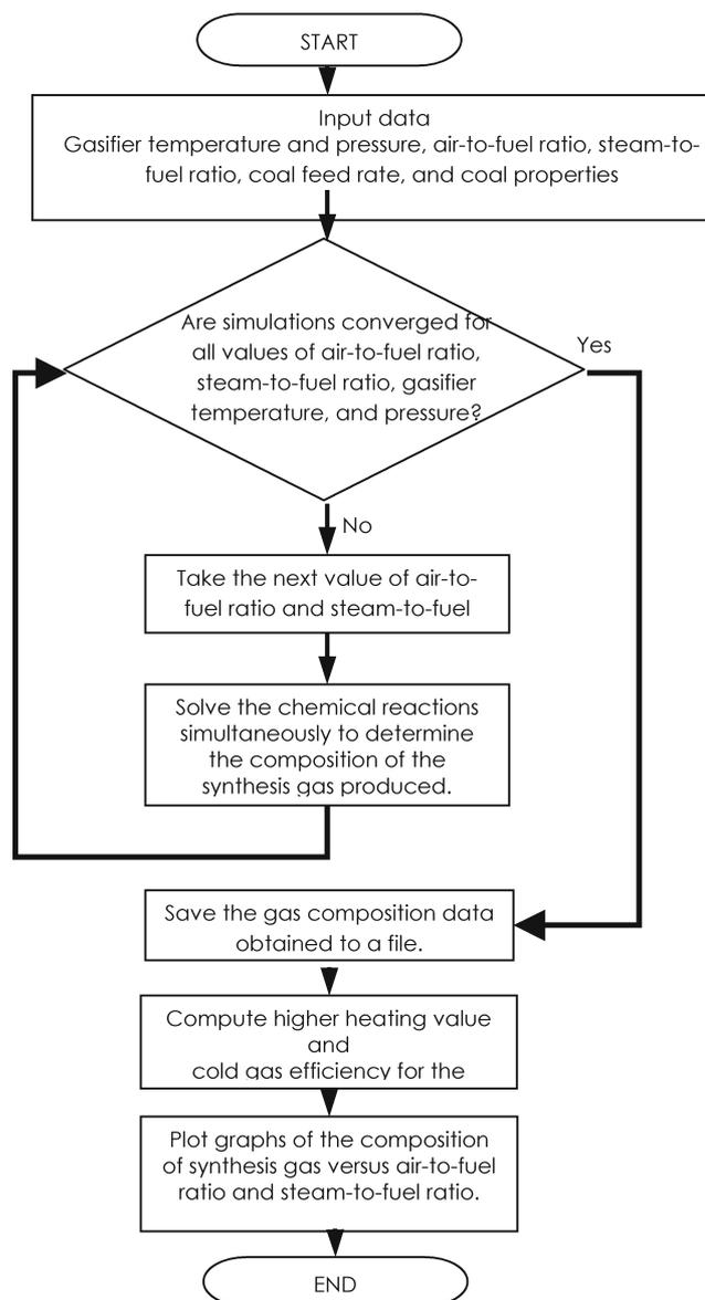
**Fig. 1.** Flow-chart of gasification model.
