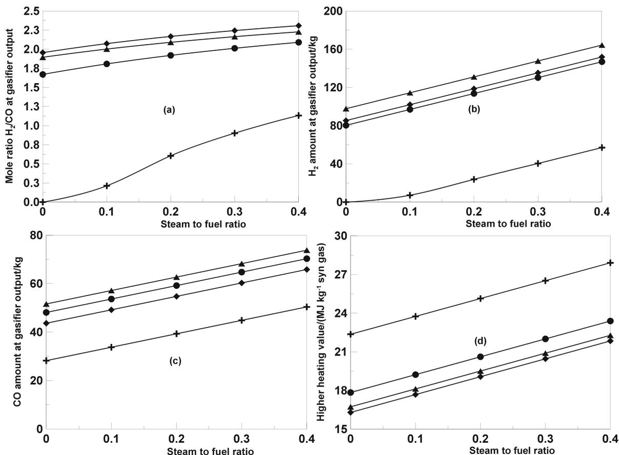
**Fig. 3.** Effect of steam-to-fuel mass ratio on  $H_2/CO$  at gasifier output (a),  $H_2$  (b) and CO (c) amounts at gasifier output, and higher heating value of syngas (d) for four different kinds of Turkish coal; ▲ – ILGIN-1, ◆ – ILGIN-2, ● – YATAGAN, + – TUNCBILEK.
