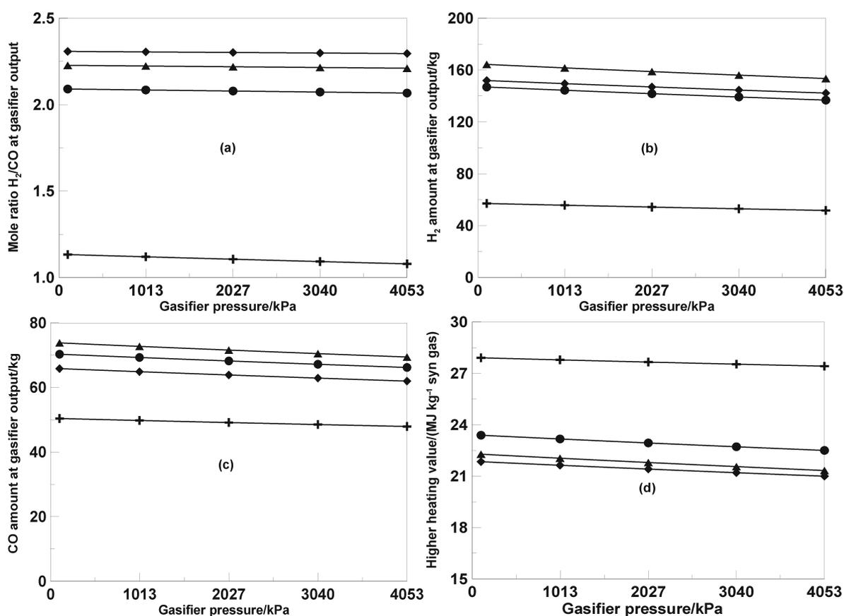
Fig. 4. Effect of gasifier pressure on  $H_2/CO$  at gasifier output (a),  $H_2$  (b) and CO (c) amounts at gasifier output, and higher heating value of syngas (d) for four different kinds of Turkish coal; ▲ – ILGIN-1, ◆ – ILGIN-2, ● – YATAGAN, + – TUNCBILEK.
