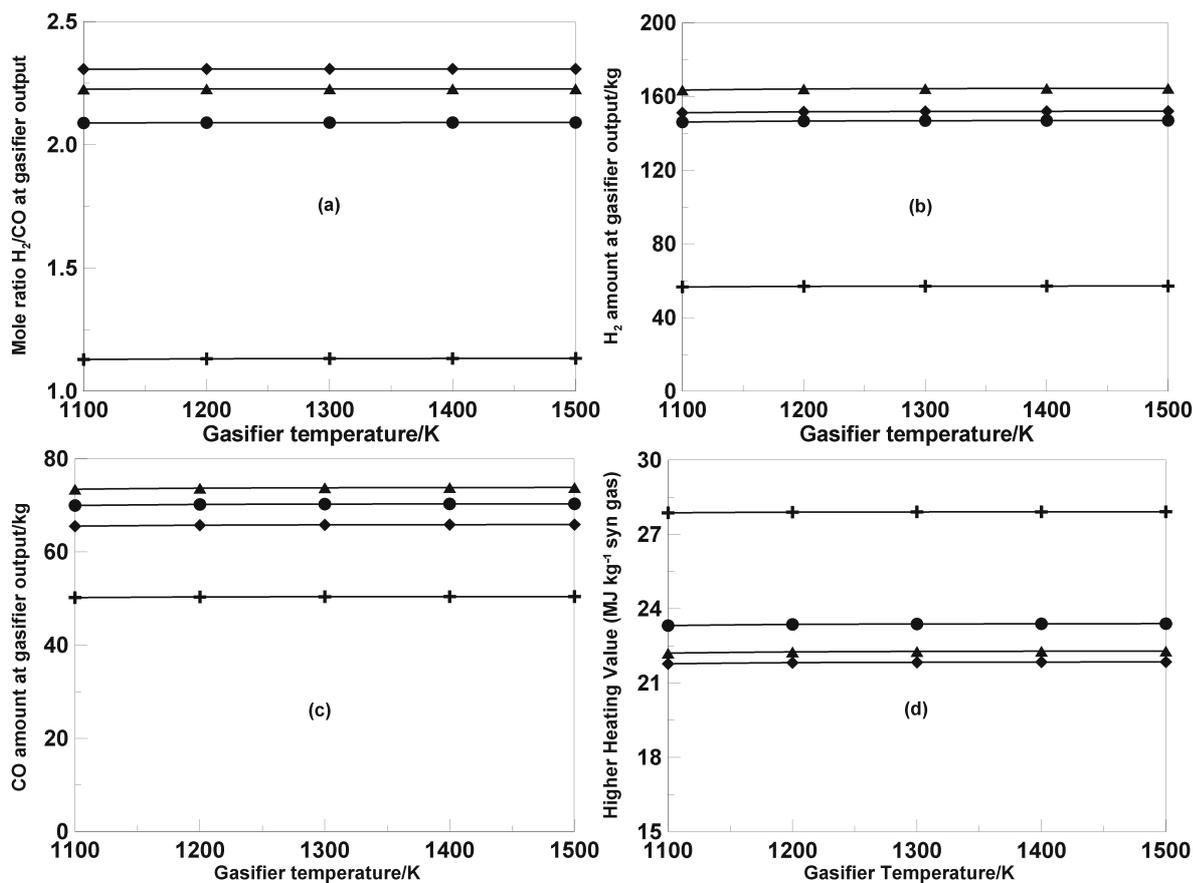
Fig. 5. Effect of gasifier temperature on H<sub>2</sub>/CO at gasifier output (a), H<sub>2</sub> (b) and CO (c) amounts at gasifier output, and higher heating value of syngas (d) for four different kinds of Turkish coal; ▲ – ILGIN-1, ◆ – ILGIN-2, ● – YATAGAN, + – TUNCBILEK.
