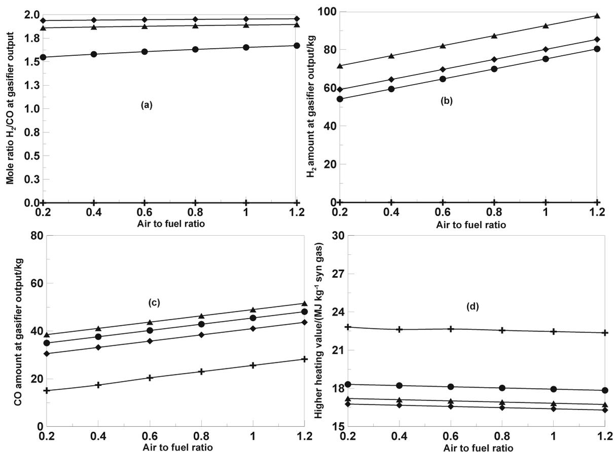
**Fig. 2.** Effect of air-to-fuel mass ratio on  $H_2/CO$  at gasifier output (a),  $H_2$  (b) and CO (c) amounts at gasifier output, and higher heating value of syngas (d) for four different kinds of Turkish coal;  $\blacktriangle$  – ILGIN-1,  $\blacklozenge$  – ILGIN-2,  $\bullet$  – YATAGAN,  $+$  – TUNCBILEK.
