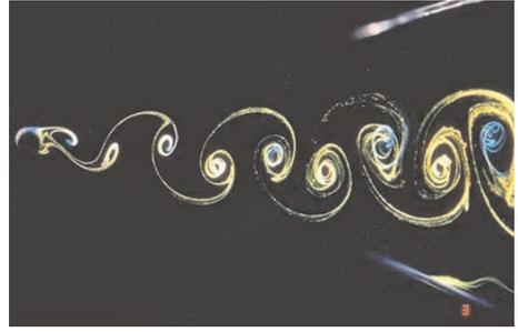
(b) Flow around a circular cylinder (figure courtesy of ONERA)
