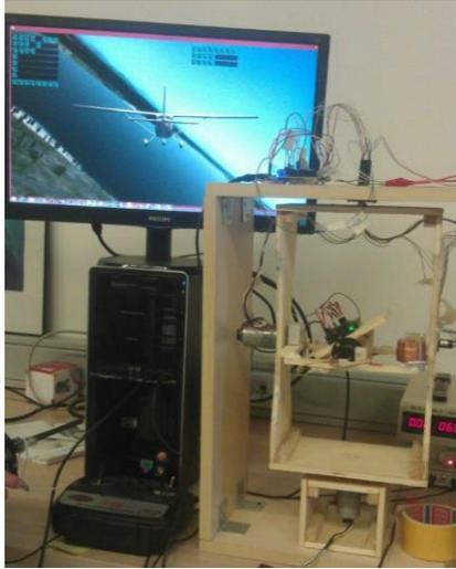
Figure 10. HIL test platform and xplane simulations
